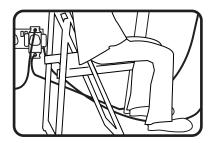
Keep cables, plugs and plugged-in equipment out of the way - it could trip you or even cause a fire!
